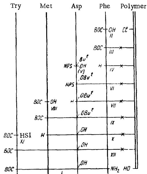
Scheme of the synthesis (conventional abbreviations for the names of the amino acids and respective groups; x represents a bond of the benzyl ester type).
